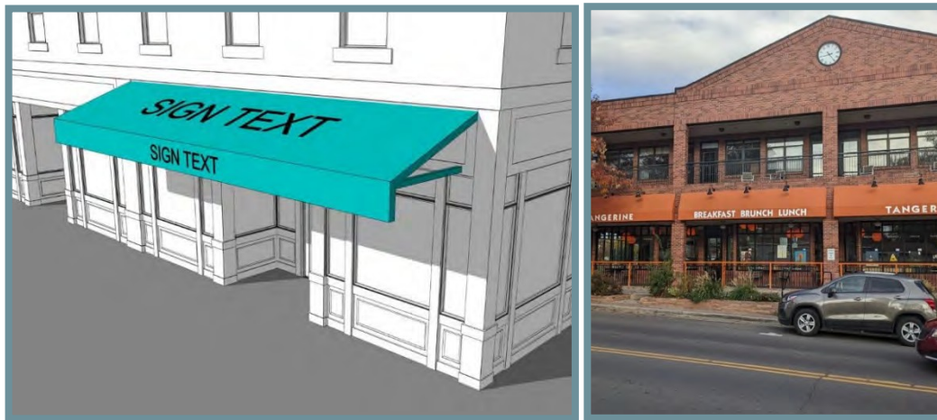
Figure 31: Canopy or awning signs--an illustration (left) and a real-world example from Colorado (right). In the image on the right, the sign text is on the valance portion of the awning (the vertical hanging portion).
