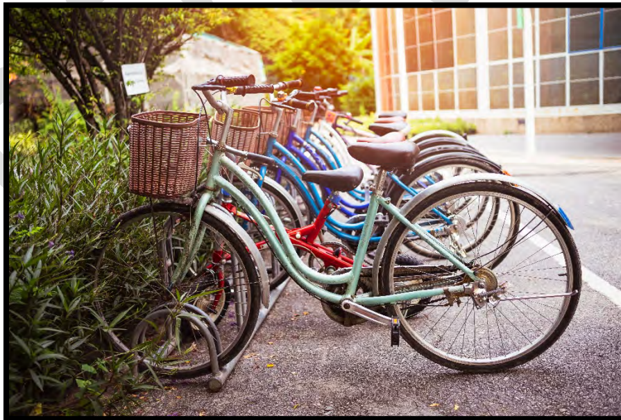
Figure 20: Image of a bike rack. This style of bike rack is not permitted to fulfill bike parking requirements per this Planning and Zoning Code as it does not allow for secure bicycle locking to the frame of the bicycle.
