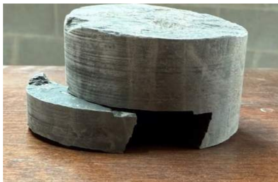
Failure Photograph of Run 3, 32.15 feet
