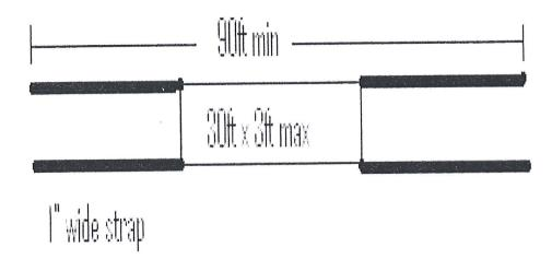
top of banner must have gromets installed at 30" centers max banner must have 2 rows of 3" wind cuts on 30" centers min
