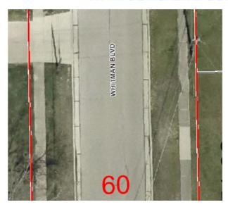
Roadway would be lowered to get positive drainage from properties onto the street and into new storm sewer where possible. If the road cannot be lowered, a yard drain would be installed.
