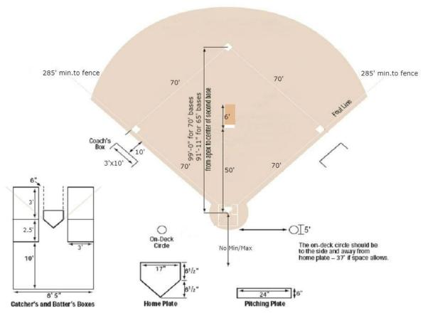
6. BATTER'S BOXES shall be provided on either side of home plate, with the inside line of this box 6 inches from home plate and parallel to the sideline. The batter's box shall be 5-1/2 feet long, extending 3 feet forward and 2-1/2 feet toward the rear, measured from the center corner of home plate. The batter's box shall be 3
